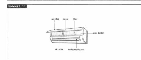
If remote controller is lost or damaged, please use aux.button to turn on or turn off the air conditioner. The operation in details is as below: As shown in the figure, open panel and press aux.button to turn off the air conditioner. When the air conditioner is turned on, it will operate under auto mode.
